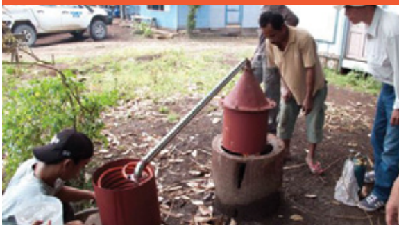
Miners in Indonesia using a mercury-capturing retort.
